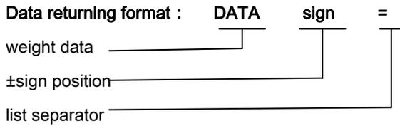
e.g.: the screen displays 31.900 , then the indicator will continuously send 009.1300 = 009.1300 = .....
